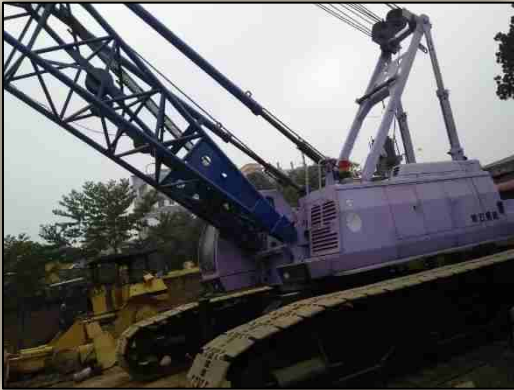
Crawler Crane 50T
